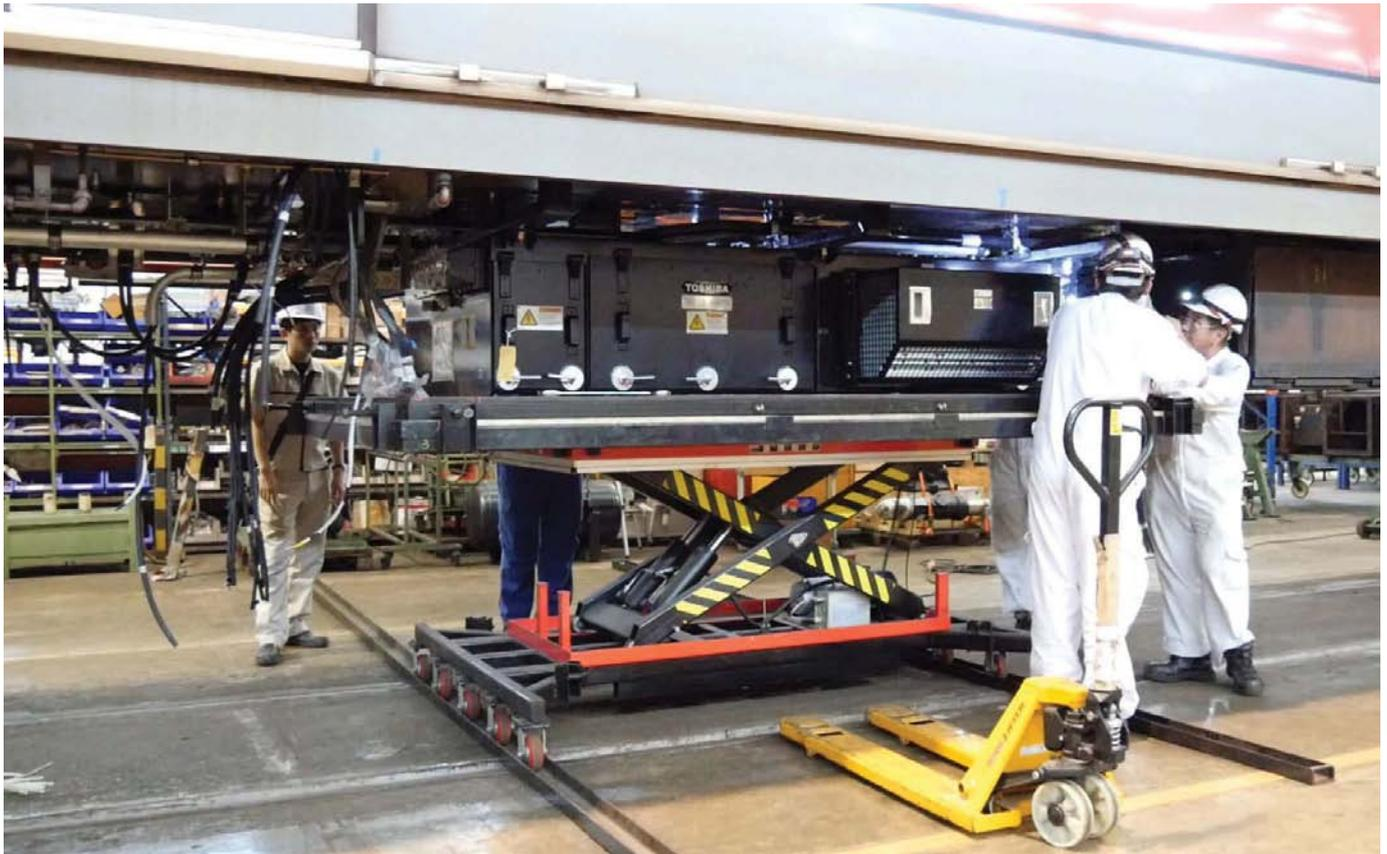
Installation of the PMSM system on a third C151 set is underway, and work on a fourth is expected to start in October.
