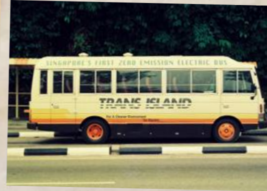
This Nissan Civilian electric bus was on trial for almost eight months
