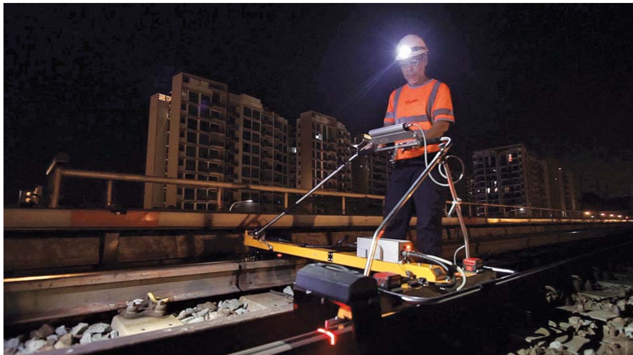
Our award-winning Laser Track Trolley allows measurement of running rail wear and track geometry to be done more safely and efficiently, while achieving high degree of reliability and accuracy.
