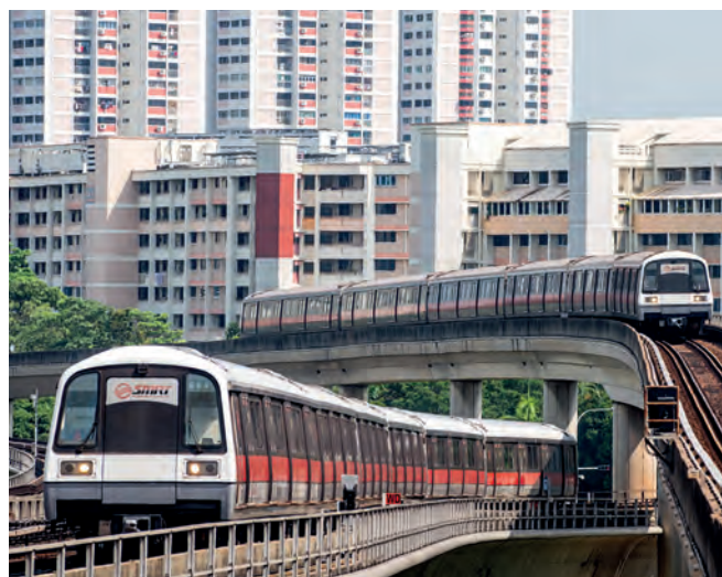
Trains employ regenerative braking to achieve savings on traction energy consumption.
