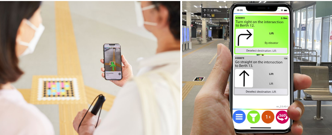
With the NaviLens app, visually impaired commuters just need to scan the tags on the floor with their mobile cameras to get information on where they are at, and find their way around a place independently.
